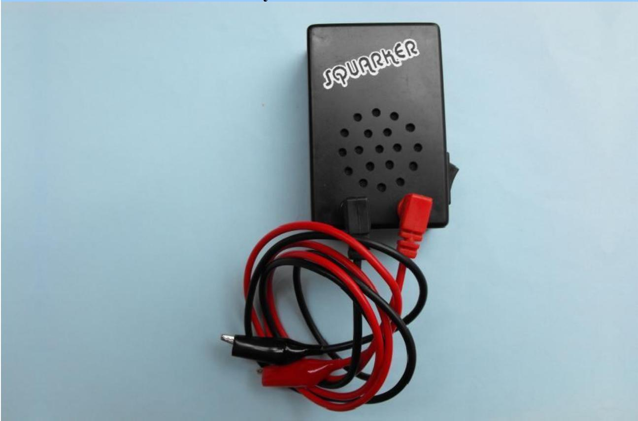
If you have ever needed to set the ignition timing on a two-stroke magneto engine, you may have had difficulty in knowing exactly when the points open. It's not something that you can easily measure, because the resistance of the coil in the magneto is quite low and there is very little difference in the resistance across the points when the points are open as compared to when they are closed.
