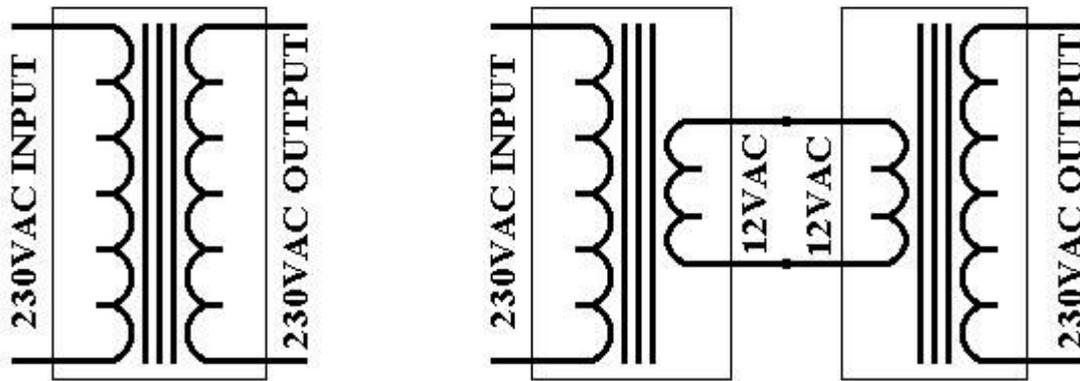
*Left: A conventional Isolation Transformer. Right: Our Isolation Transformer.*
