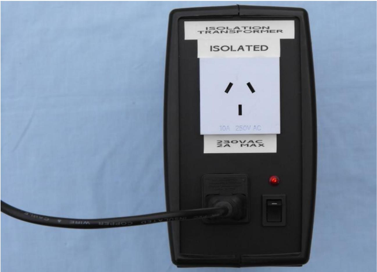
*Above: The back panel of the Isolation Transformer showing the sockets & switch.*
