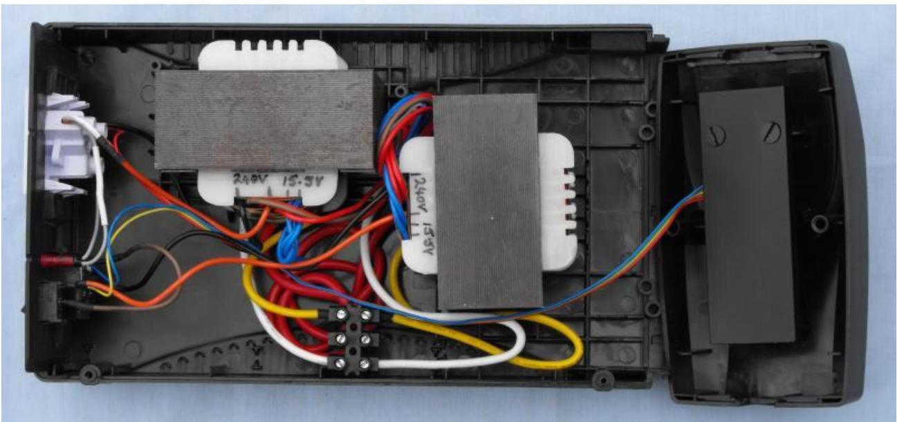
*Above: The layout inside the prototype Isolation Transformer.*
