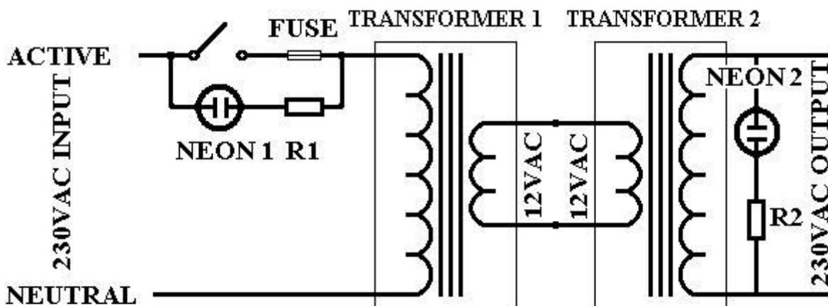
*Above: This is how the transformers and other components are wired up.*
